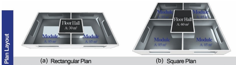
Figure 2. Plan layout alternatives: (a) rectangular plan with 2 modules; (b) square plan with 4 modules.
